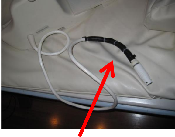
Coil with plastic tubing and zip ties used to cover damaged cable
